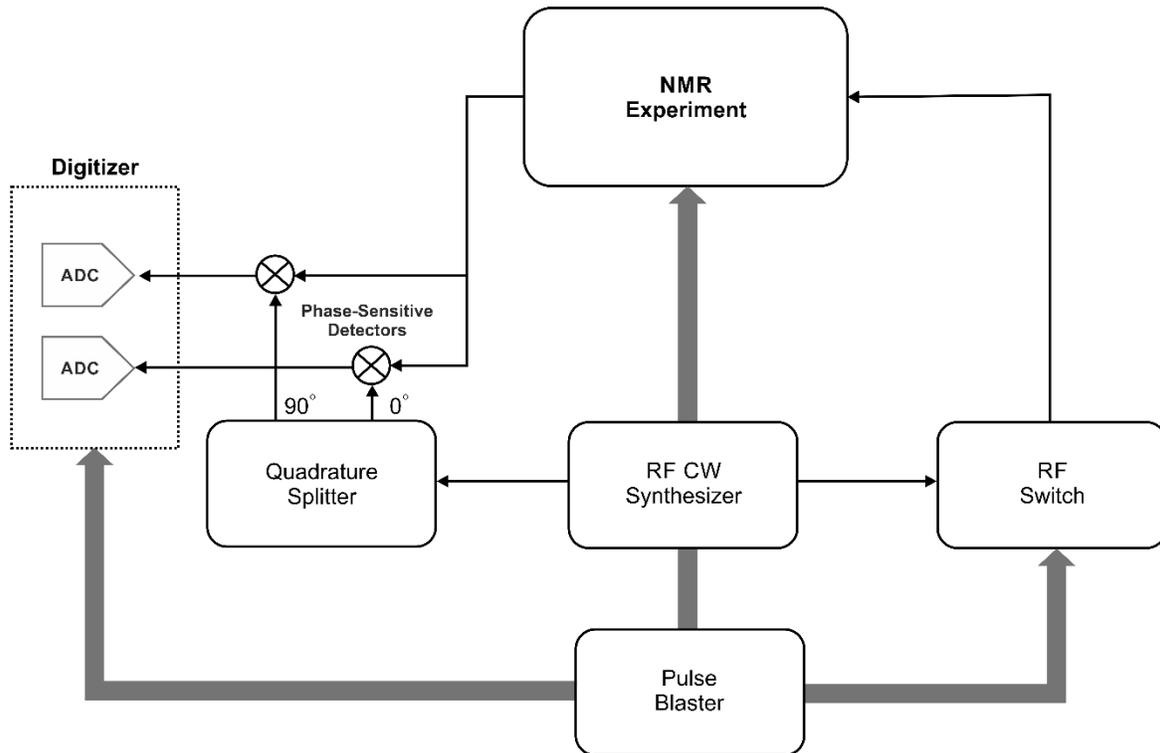
**Figure 2.3 Traditional FID Complex Waveform Acquisition**
