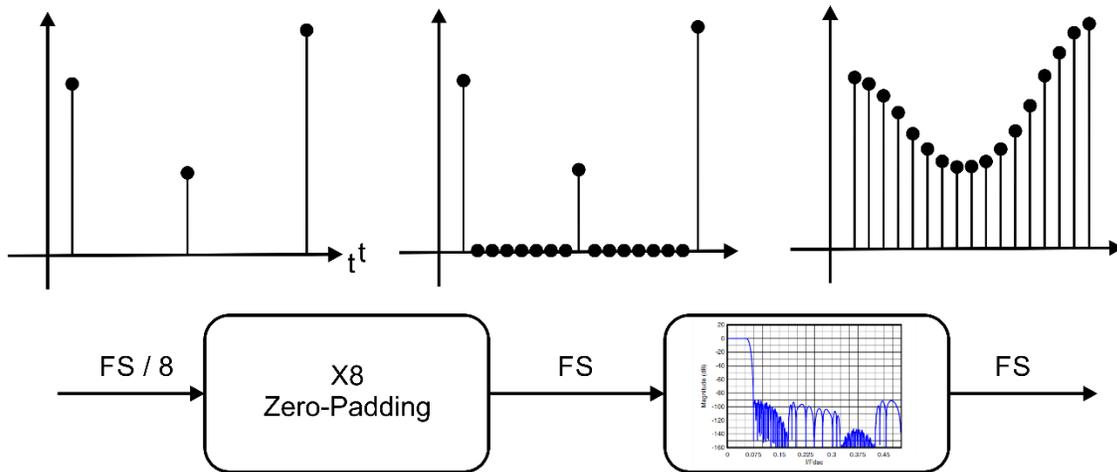
**Figure 2.2 Real Time Interpolation of the Pulse Envelope Waveform**
