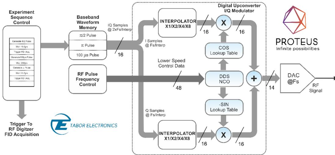
**Figure 2.1 Proteus AWG Channels Block Diagram**
