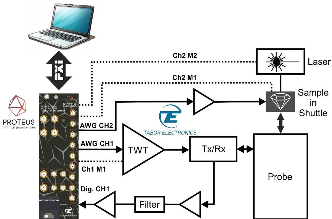
**Figure 1.1 Proteus AWT Integrated in an NMR System**
